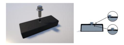
Proper tightening of the V-MAG© bolts is important to protect the V-MAG© from potential corrosion and a reduced lifetime. Secure the bolts properly by tightening the bolt shoulder against the rubber surface of the V-MAG© and create a sufficient seal.
