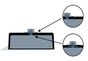
Proper tightening of the V-MAG© bolts is important to protect the V-MAG© from potential corrosion and a reduced lifetime. Secure the bolts properly by tightening the bolt shoulder against the rubber surface of the V-MAG© and create a sufficient seal.
