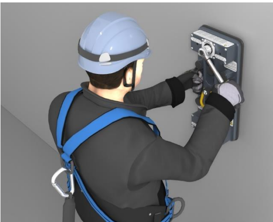
Release both Thrust Leg Hex Head's
