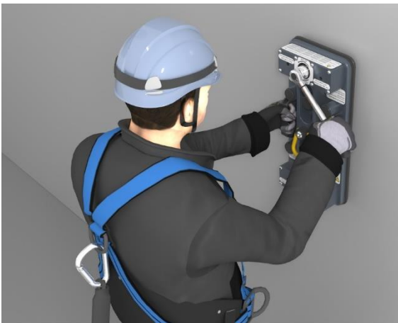
Release both Thrust Leg Hex Head's
